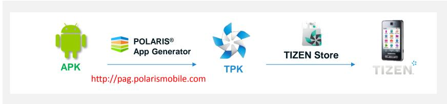
\* Android APK is automatically converted to TIZEN TPK, which can be uploaded to TIZEN store, downloaded into TIZEN device, and executed as same as TIZEN app
